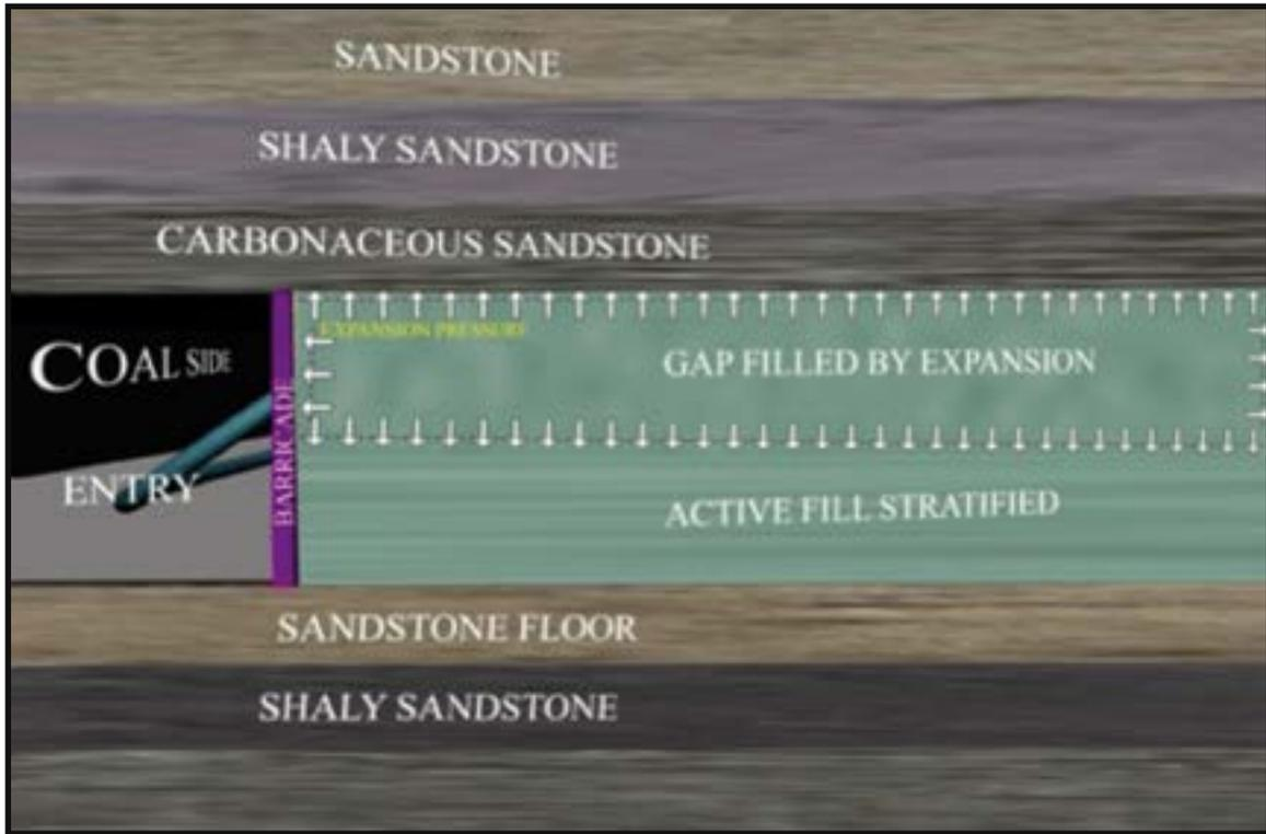
Fig. : 5 : Paste in the Slice under Expansion and Setting Solid Simultaneously
