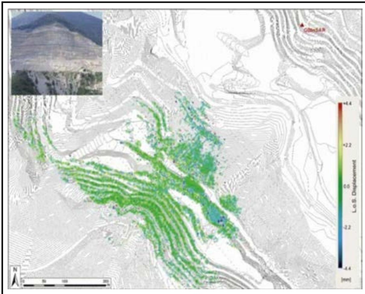
*L.o.s. Displacement Map of a Quarry Rock Face in NW Italy recorded from 28 June to 7 July, 2011.
