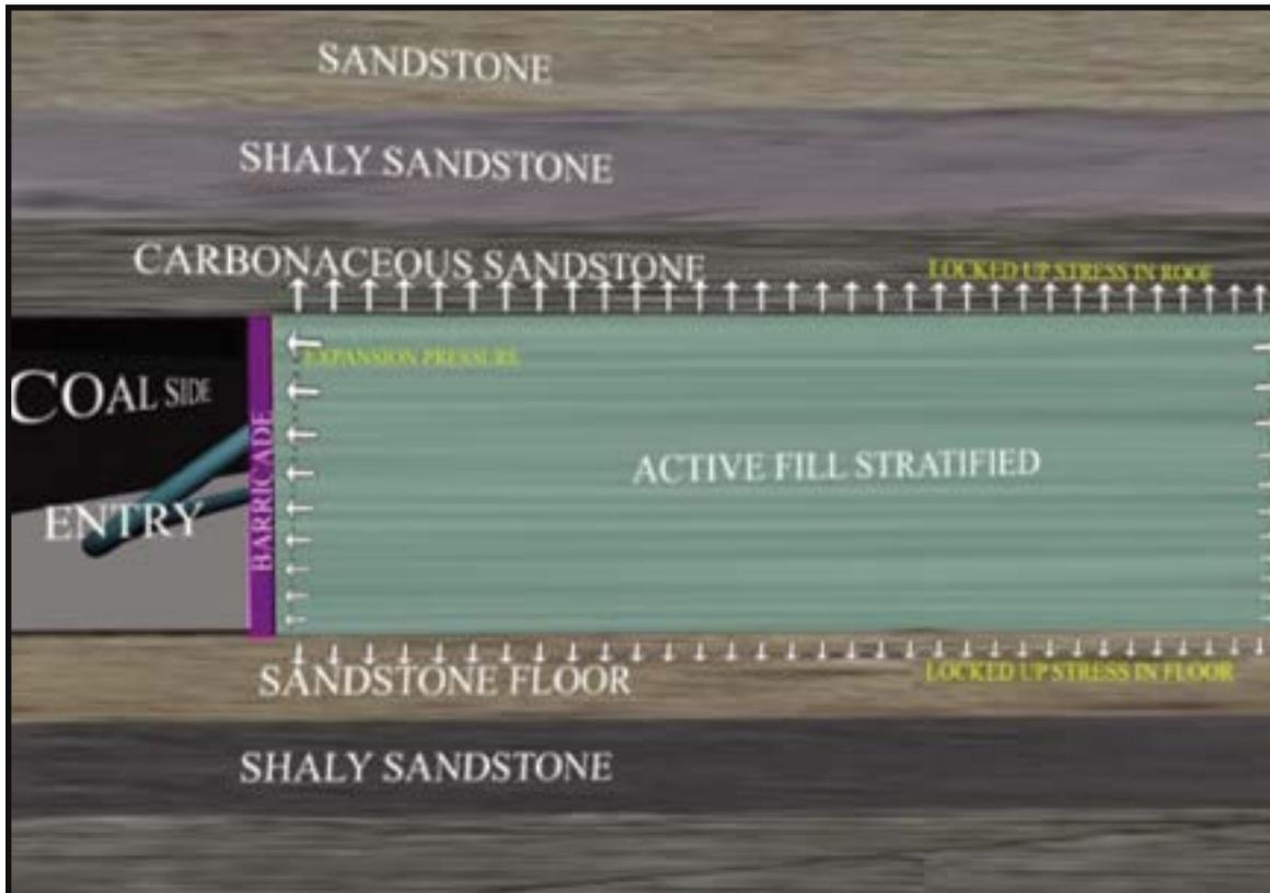
Fig. : 6 : AFM solidified and stresses locked up
